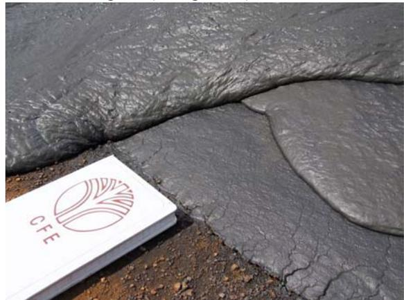
Photo 4: Three thin layers of paste tailings.
