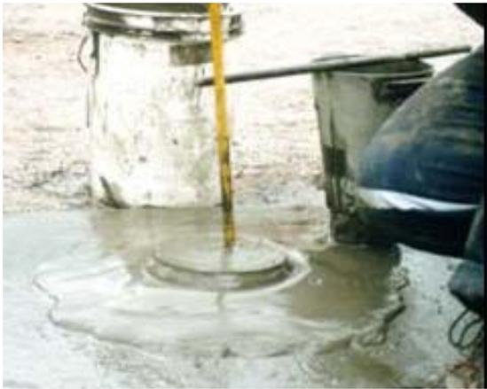
Photo 1: 250 mm (10 in) slump paste tailings.
