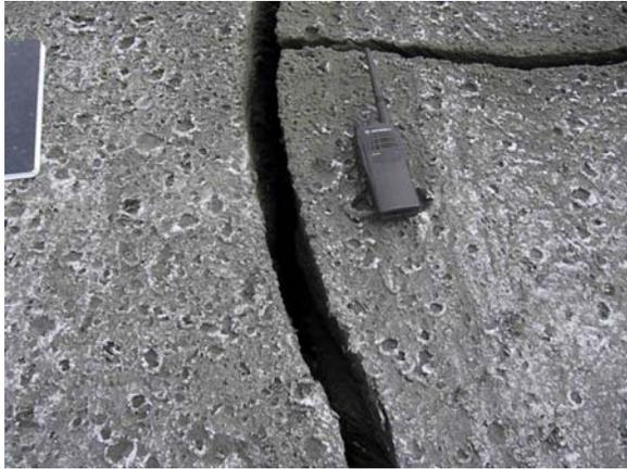
Photo 9: Wide desiccation crack in thickly deposited tailings layers (about 4 month old deposition).
