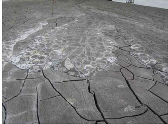
Photo 10: Thin layer of tailings deposited over heavily desiccated thickly deposited tailings.
